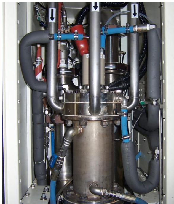
Fig. 4: decentralised exhaust air purification system
