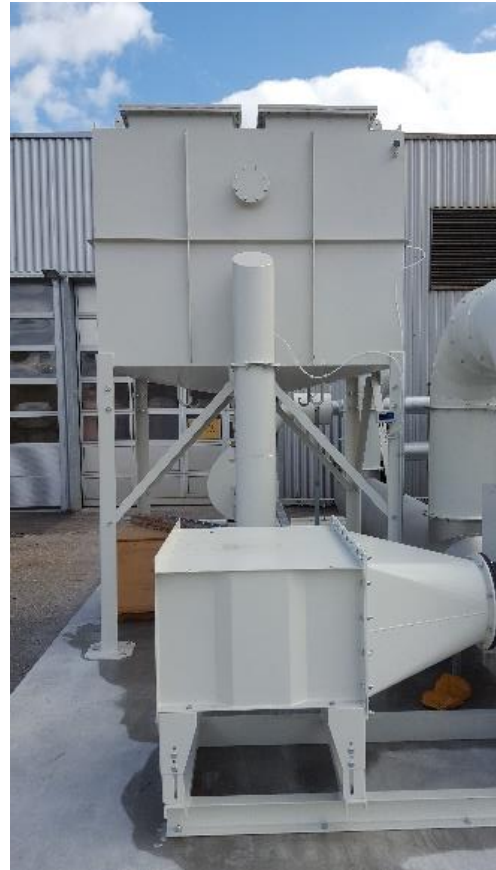
Fig. 1: Activated carbon filter for odour reduction for max. 2.500 m 3 h raw gas
