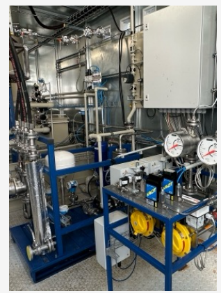
2 x 50 kW CFC decomposition in chemical industry
