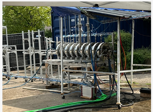
Technology demonstration reactor for methane pyrolysis
