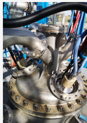
Conditioning of pyrolysis gas
