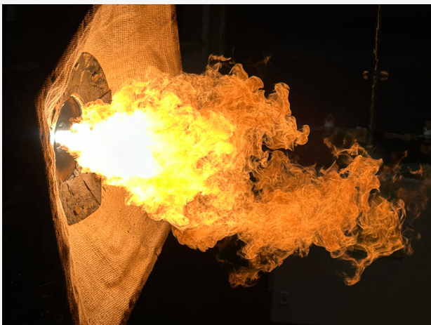
100 kW hollow cathode torch with 100 % methane as plasma gas
